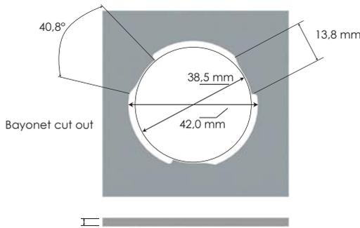
Wall thickness for bayonet version : 2,0 mm ± 0,2 mm
